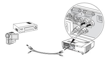
2. Connect the other end of the cable to the audio output connector(s) on your computer or video equipment.
