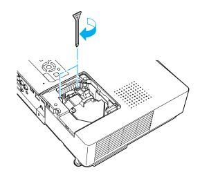
Replace the lamp cover, then tighten its screw. 8.
