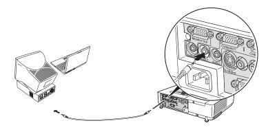
■ If you have equipment connected to the Video or S-Video port, connect an RCA-style audio cable to L-Audio-R.
