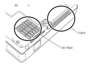
3. If the dirt is difficult to remove or the filter is broken, replace the filter as described on page 177. Contact your dealer or call Epson at 800-GO-EPSON (800-463-7766) to obtain a new filter.
