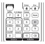
While holding the ID button, press a numbered button on the remote control (0 through 9) to select the desired ID. Select zero to control all projectors, or select a number to match the ID of the projector(s) you want to operate.
