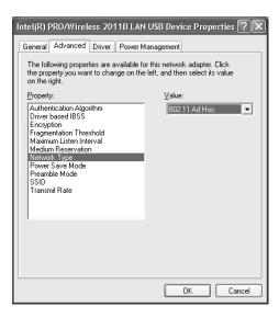
When you connect in Ad Hoc mode, your connection to other wireless networks or devices is broken. If you need to remain connected to your wireless network, use Access Point mode, as described on page 68. Also, make sure you reconnect to your original wireless network when you are done using the projector.
