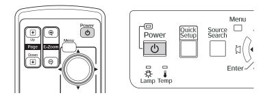
The projector beeps once and the **Power** light flashes green as the projector warms up, then an image begins to appear. When the **Power** light stops flashing and remains green, the projector is ready for use.
