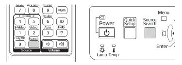
You can also use the **Source** buttons on the remote control to switch between devices connected to the ports identified on each button, or select EasyMP<sup>®</sup> to project wirelessly or from a USB drive.
